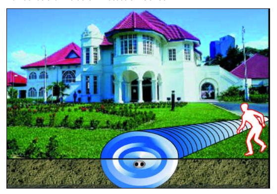
Perimitrax<sup>®</sup> is a covert perimeter intrusion detection sensor that generates an invisible electromagnetic field around buried sensor cables. If an intruder disturbs the field, an alarm is declared. In the case of a network system, the alarm is instantly communicated over the sensor cables to a PC-based central control system.
